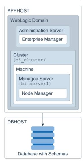
Figure 1-1 Oracle Analytics Server Standard Installation Topology
