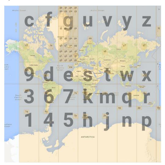
Figure 10-5 Level-1 and Level-2 Geohash Cells
