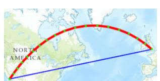
Figure 10-1 Geodetic vs Straight Line
