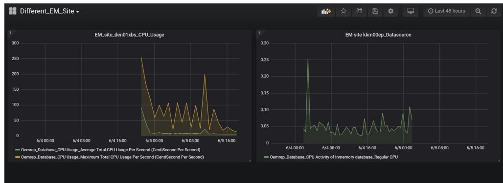
Dashboard with a single panel pulling data from a different Enterprise Manager sites (Data from multiple Enterprise Manager sites , single panel):
