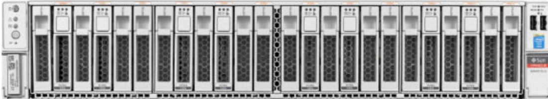
Figure 3-21 Front View of Extreme Flash Exadata Storage Server X5-2 Servers
