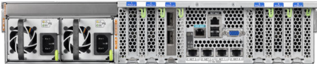
Figure 3-22 Rear View of Extreme Flash Exadata Storage Server X5-2 Servers
