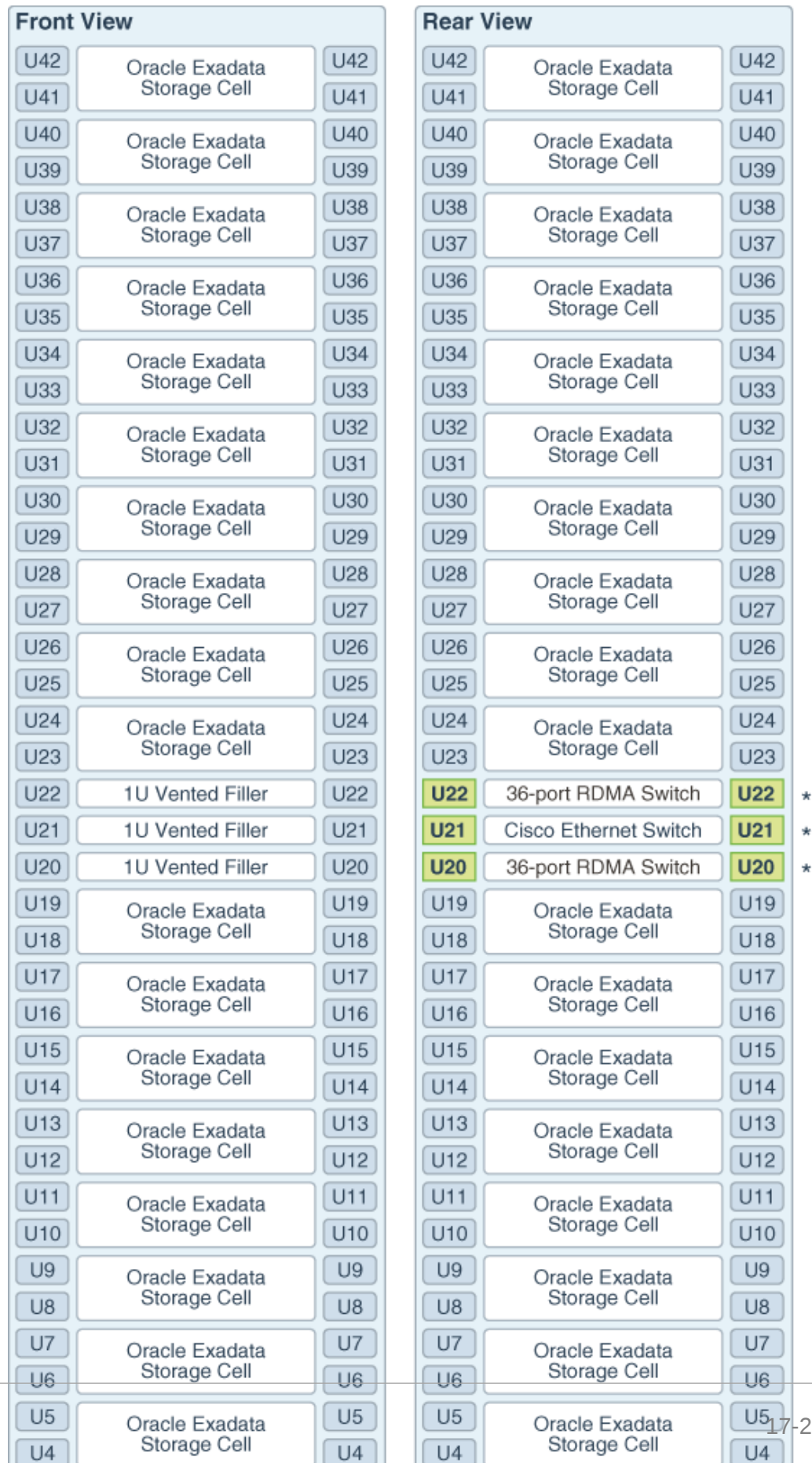
Figure 17-1 Rack Layout of Oracle Exadata Storage Expansion Rack X9M-2
