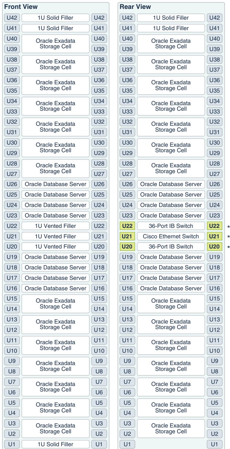
Figure 12-1 Rack Layout of Oracle Exadata Database Machine X8-2 and X7-2 Full Rack
