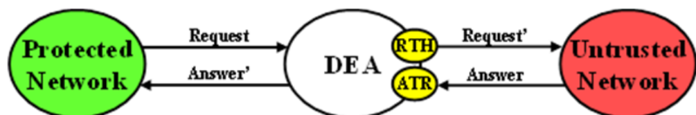
Figure 10-2 Diameter Topology Hiding Trigger Points: Protected-to-Untrusted Transactions
