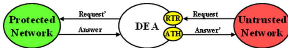
Figure 10-3 Diameter Topology Hiding Trigger Points: Untrusted-to-Protected Transactions
