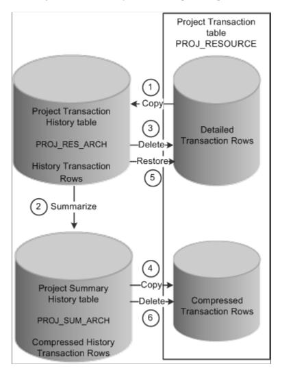
The data compression and restoration process flow that the system performs is:
