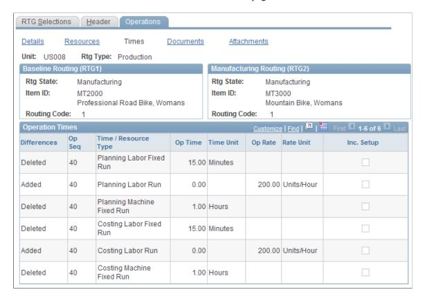
This page displays differences in operation sequences, time or resource types, operation times, time units, operation rates, and rate units. It also indicates whether the time is included in the setup.
