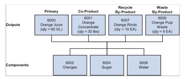
When used on a multiple-output BOM, the BOM quantity represents the in-process quantity for the BOM item as a batch item (as opposed to the item ID as a primary item). For example, if the example BOM structure has a BOM quantity defined as 150, then the in-process units of the batch are 150.
