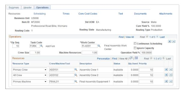
The page displays differences in operation sequence, resource types, crews, machines, tools, quantity used, and priority.
