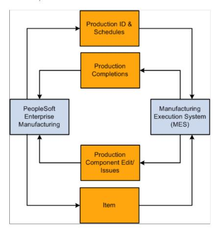
You'll continue to use PeopleSoft Manufacturing for planning, material movement into WIP, validation of completion data, and production costing functions. PeopleSoft is the system of record for setup information, including item masters, bills of material, routings, and creating production orders.
