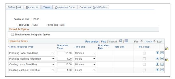
Task times are divided into labor and machine setup, run, fixed run, and post production. Additionally, you can have separate sets of times and run rates for planning and costing purposes. You can define intransit and queue time for planning purposes only. When defining time and run rates, define only the types that apply to the task.
