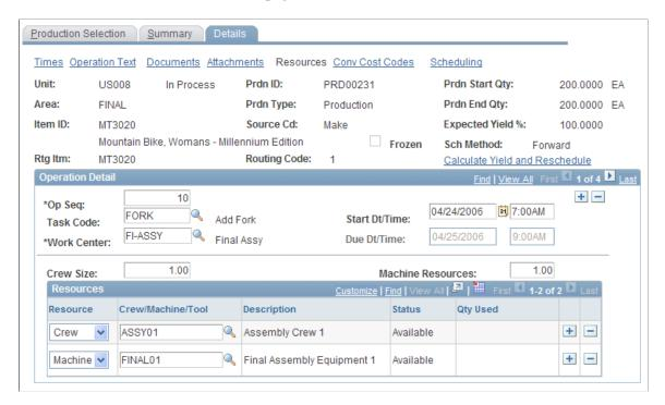
When maintaining the operation list, you can optionally define the crews, machines, and tools that will be used at work centers to perform specific tasks. In addition, keep these in mind when maintaining operation resources:
