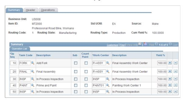
The operation sequences defined here correspond to the operation sequences that you specify for components on the item's BOM. If you have not assigned operation sequences to the item's BOM and you want to issue a component to the operation's WIP location, return to the BOM Maintenance component after you have added the item's routing.
