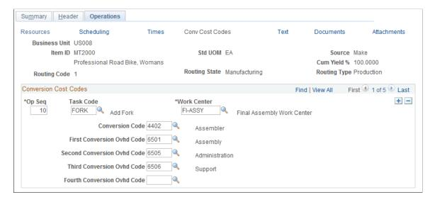
Conversion cost codes determine the labor, machine, outside processing, and overhead cost of the operation. When defining the costs, you associate a conversion rate or cost to each conversion code. The code is then entered on the task or work center, depending on the manufacturing installation options. The system then associates the corresponding rates with the operation when it copies the task or work center to the routing or operation list.
