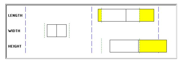
The left and right edges of the capability graph box represent the plus and minus 3 sigma values, and the centerline represents the mean value. In addition, green dashed lines represent the lower-and upper-specification limits, while yellow parts represent the areas out of specification based upon the distribution fitting (Normality, Pearson Best Fit) criteria in effect.
