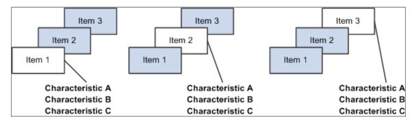
Using the by subgroup method, you inspect one characteristic for a group of items, then another characteristic for a group of items, such as inspecting several small items in succession with a specific gauge. You complete the sample for each characteristic prior to using the next gauge.
