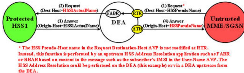
**Figure 9-14 S6a/S6d HSS TH Untrusted-MME/SGSN to Protected-HSS Transaction**
