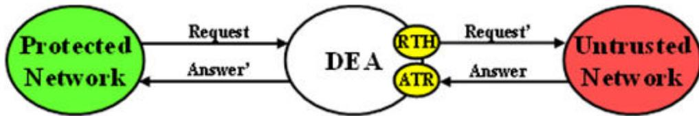
For Untrusted-to-Protected Network Diameter transactions, any topology-hidden information embedded in the Untrusted-to-Protected Network Request message may be a candidate for topology information restoral. The Trigger Point for evaluating whether topology-related information in a Request message should be restored is called Request Topology Restoral (RTR).
