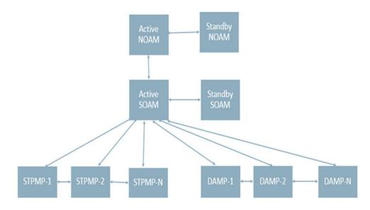
Figure 2-7 STP-MP and DA-MP in a Site
