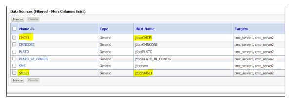
Once the Data Sources are mapped with the corresponding DB schemas and servers, restart the PLATO, CMC, SMS, and other required managed servers.
