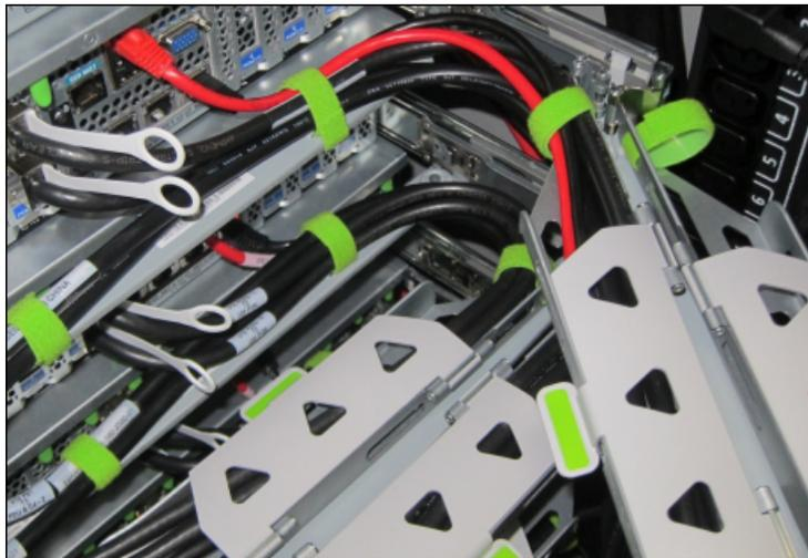
4. Close the crossbar covers to secure the cables in the straightaway.
