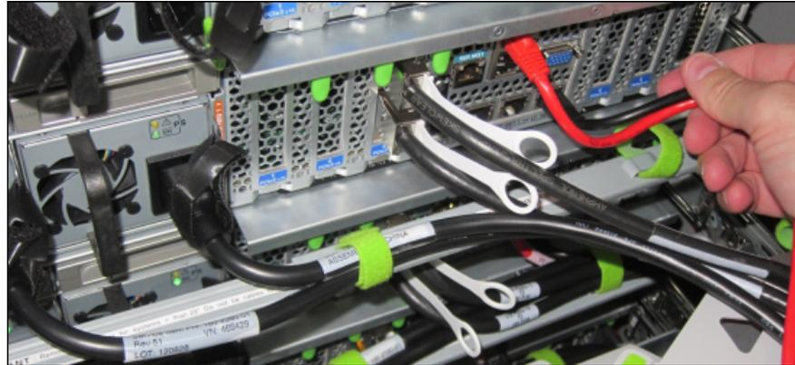
3. Route the cables through the CMA and secure them with hook and loop straps on both sides of each bend in the CMA.
