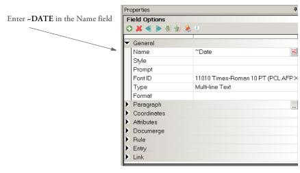
No other rules or script calculations are required. During print processing, each time the section that contains this field prints, the system will assign a date value.
