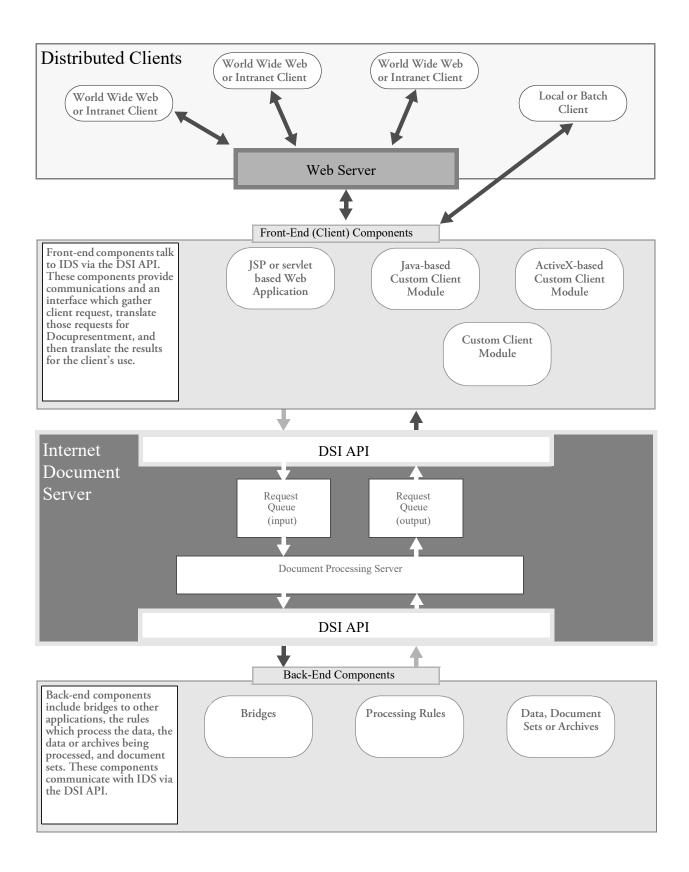
Two-tier and three-tier models are supported. In the three-tier model, the remote client can take a variety of forms and paths. The remote can be a web browser using CGI, a web browser using Java, or stand-alone, *fat* or *thin*, Java or C clients. Notice that there are two paths from the remote client, one through a front-end component, such as CGI, JSP or servlet, and the other through a Java client. The two paths merge at the DSI API, one for C the other for Java.
