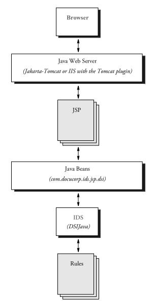
The name *REQTYPE* is reserved for the request type to the IDS rule. Once the request name/value has been passed to the dsi JavaBean, ProcessRequest is called to send the name/value and request type to the IDS rules.
