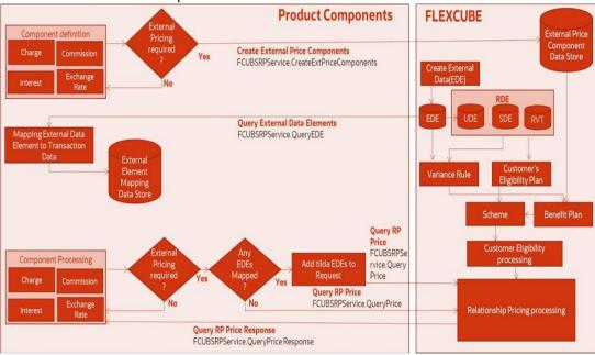
Above diagram depicts the high level interactions between the banking product components and FLEXCUBE RP module to support external pricing.
