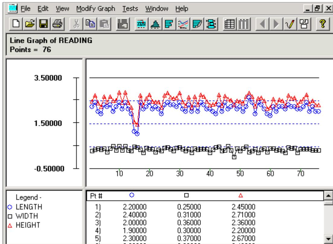
The line graph comprises multiple graph panes (sections) displaying information about the subset that you are examining. All subsets that you are comparing are overlaid on the same graph. You can select individual points on the line graph display to examine details.
