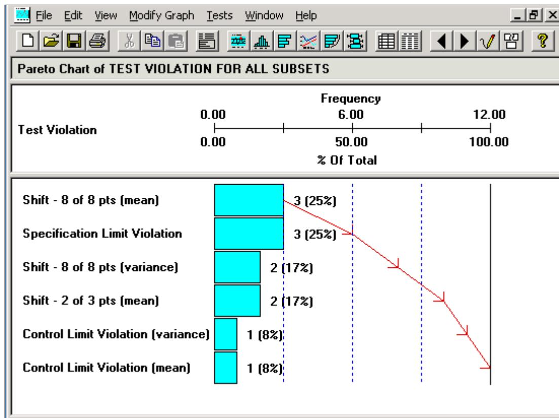
A Pareto chart is comprised of multiple graph panes (sections) and includes information about the subset that you are examining. You can resize the sections the same way that you resize histogram sections.
