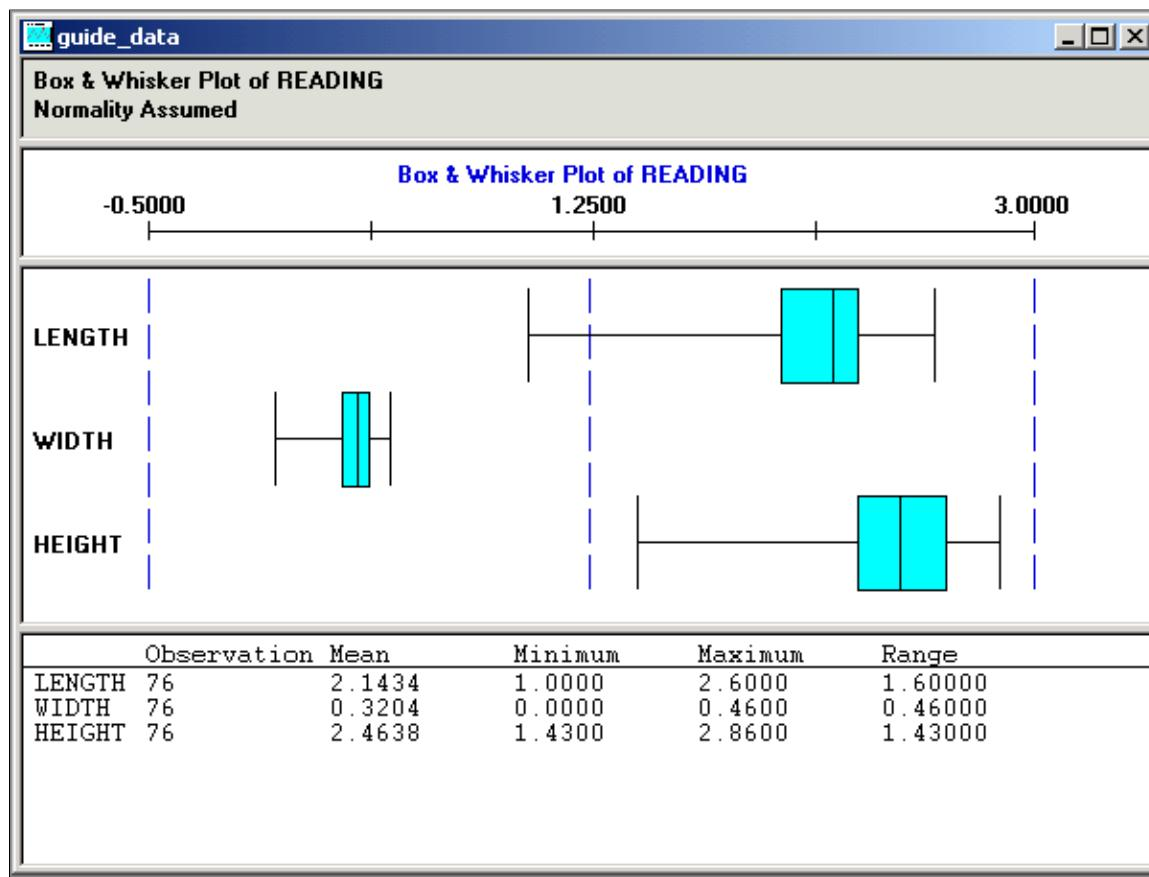
The box plots display is comprised of multiple graph panes (sections), with each section displaying information about the subset that you are examining. Box plots are also referred to as Box and Whisker plots, because of the vertical whisker lines at each end of the horizontal scale.
