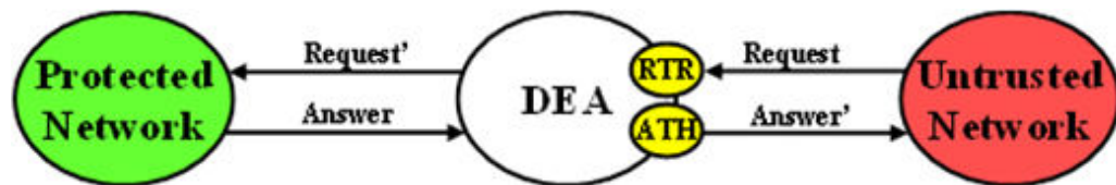
Figure 9-3 Diameter Topology Hiding Trigger Points: Untrusted-to-Protected Transactions
