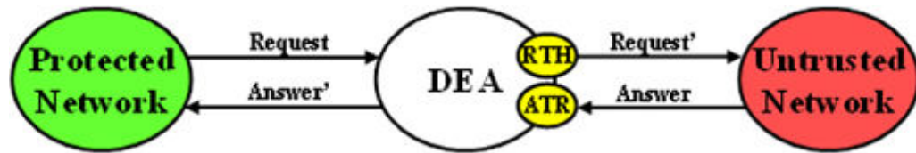
Figure 9-2 Diameter Topology Hiding Trigger Points: Protected-to-Untrusted Transactions
