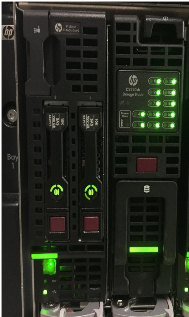
Figure 4. BL460C Gen 9(with storage array) Layout
