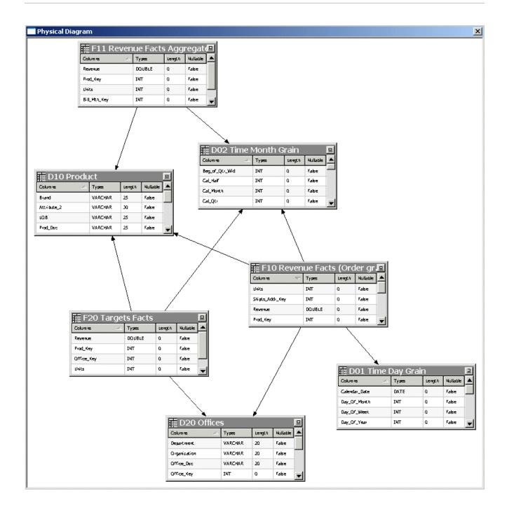
You can also open the Physical Diagram by selecting one or more objects in the tree view and clicking the **Physical Diagram** button on the toolbar:
