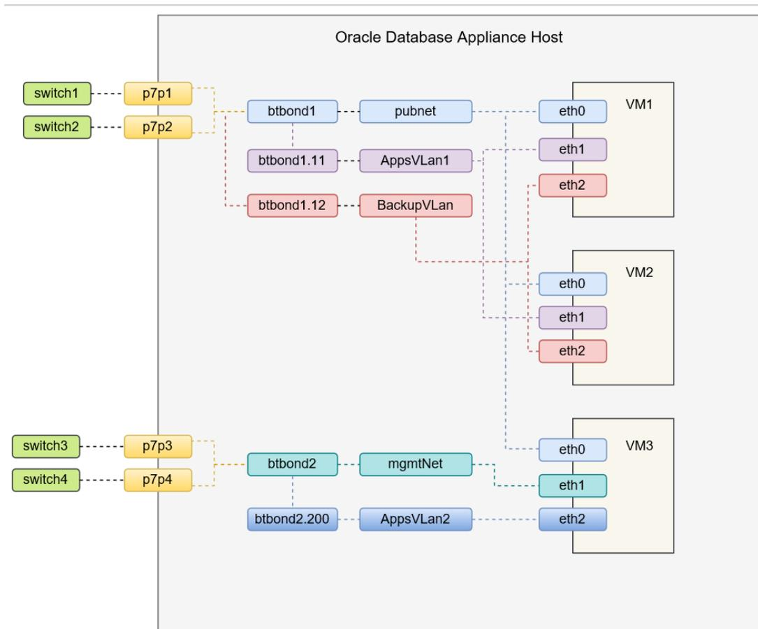
Oracle Database Appliance KVM virtual network supports two type of networks, bridged and bridged-vlan. The above figure is an example of the KVM virtual network on Oracle Database Appliance X8-2 hardware models.
