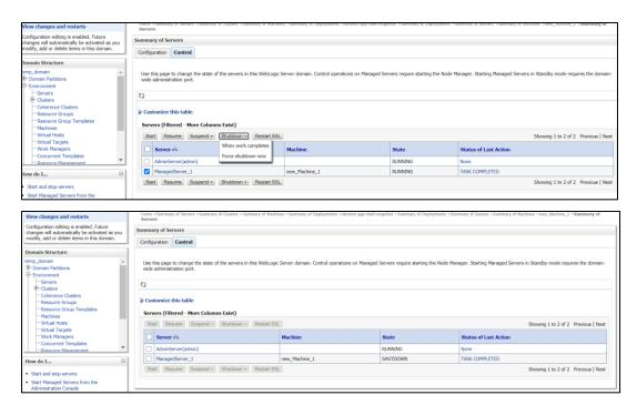
3. Once shutdown is completed, navigate to **Control** and select the servers to start and confirm action.
