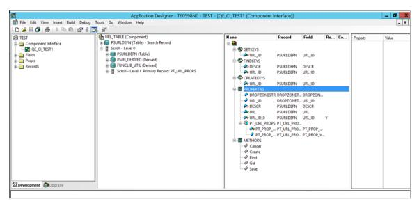
Similar to other component interface properties, the records and fields from the custom subpages can be retrieved to be modified or deleted directly, or through component interface collections.
