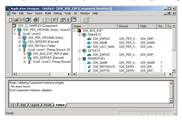
The component view shows records and scrolls in the component, using a tree representation. The structure is the same as the one you see on the structure tab of a component in PeopleSoft Application Designer. Drag the fields and collections that you want exposed to the component interface view.
