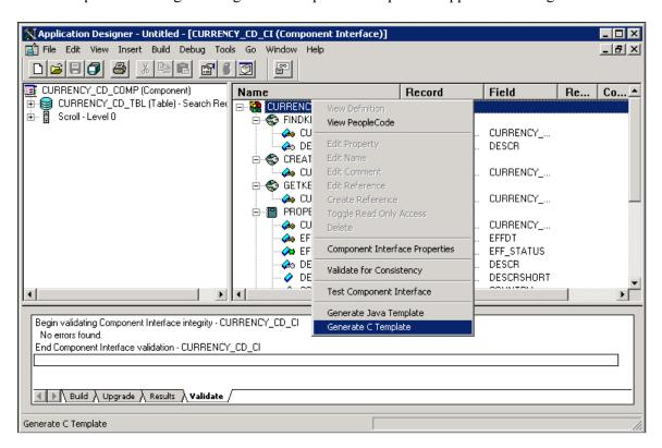
To generate a C++ template for a component interface:
