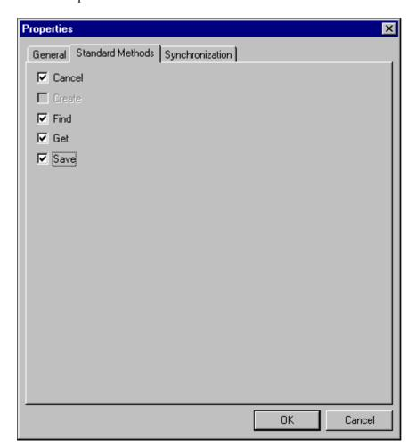
Use the Properties – Standard Methods tab to enable or disable standard methods.
