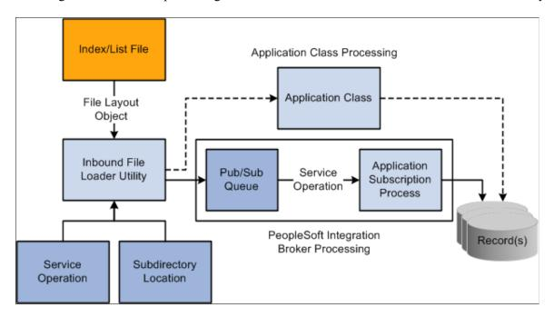
The flow for inbound file processing using the Inbound File Loader utility is:
