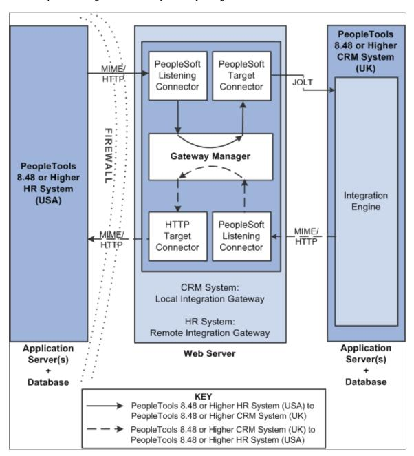
For this configuration scenario, one PeopleSoft application and one integration gateway reside on each side of the firewall. The integration gateway can reside on the same physical machine on which you have installed the PeopleSoft application, or it can reside on its own machine.
