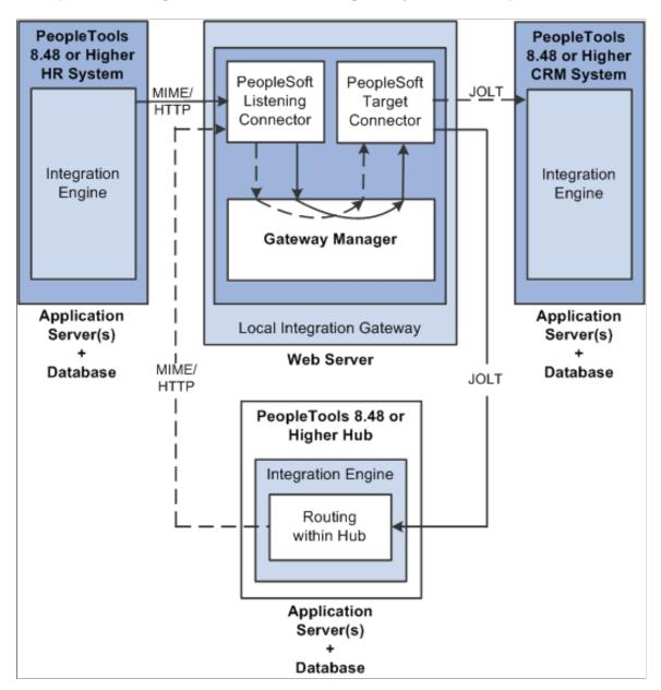
In this scenario, all of the routing rules and transformations are located on the hub.
