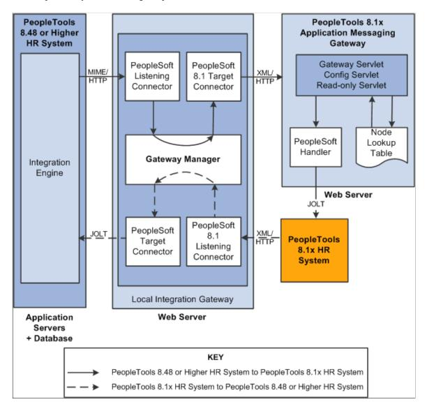
In this scenario, you must configure the PeopleSoft Integration Broker system, the integration gateway, and the PeopleTools 8.1x system. The remainder of this section highlights these tasks by using the systems and components shown in the diagram as examples.
