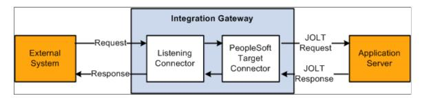
After the incoming request has been received by the integration gateway, the flow through PeopleSoft Integration Broker is the same, regardless of the listening connector used. With this in mind, no specific listening connector will be discussed here. The scenario is simple: a request is sent into the gateway, which then passes it on to the application server. The application server processes the request, and returns a response.
