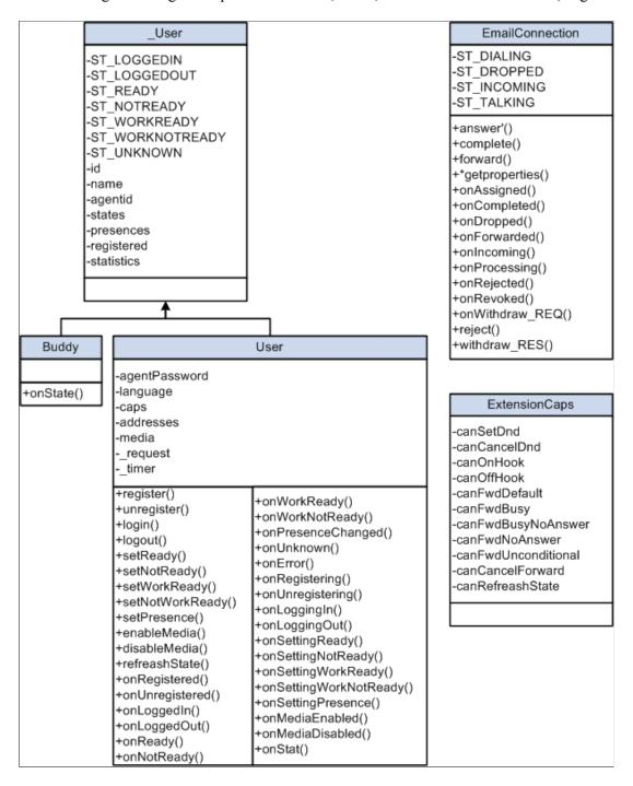
The following class diagram explains the classes, fields, and methods of JSMCAPI (diagram 3 of 4).
