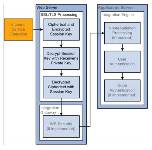
When the service operation arrives on your web server, it is one package that contains the ciphertext (encrypted service operation contents) and the encrypted session key that decrypts the ciphertext.
