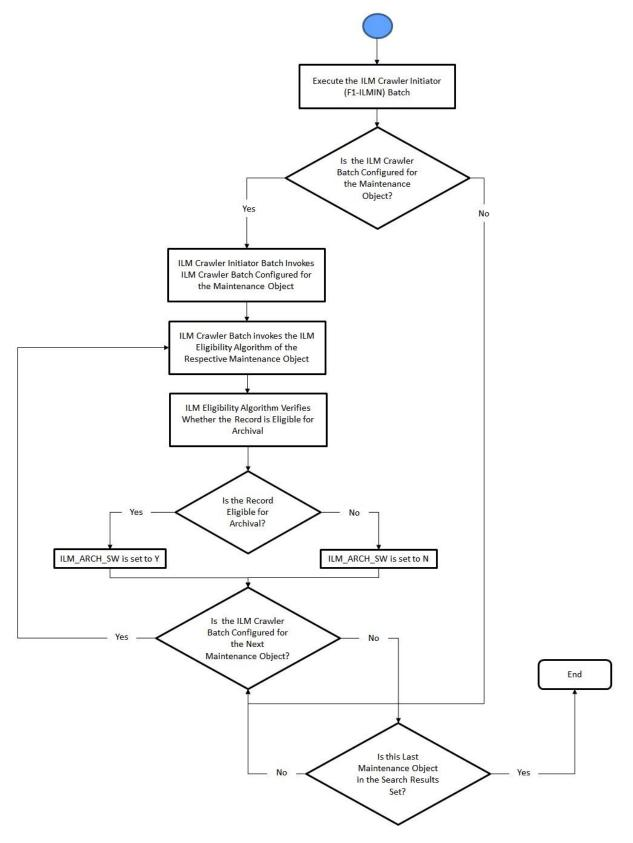
Figure 3: ILM Crawler Initiator Batch Execution Process
