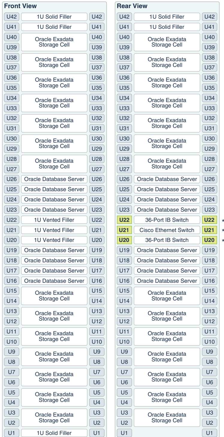
Figure 13-1 Rack Layout of Oracle Exadata Database Machine X8-2 and X7-2 Full Rack
