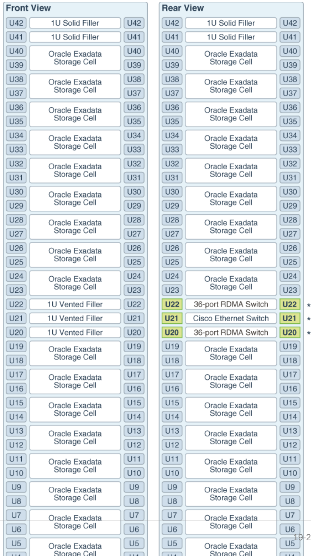
Figure 19-1 Rack Layout of Oracle Exadata Storage Expansion Full Rack X5 to X8M
