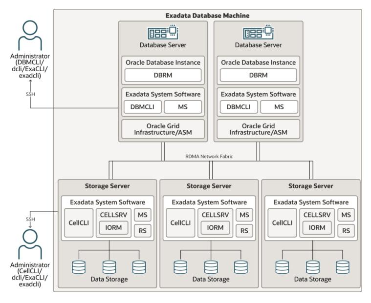
Oracle Exadata System Software provides database-aware storage services, such as the ability to offload SQL and other database processing from the database server. The database and storage servers both contain components of the Exadata System Software.
