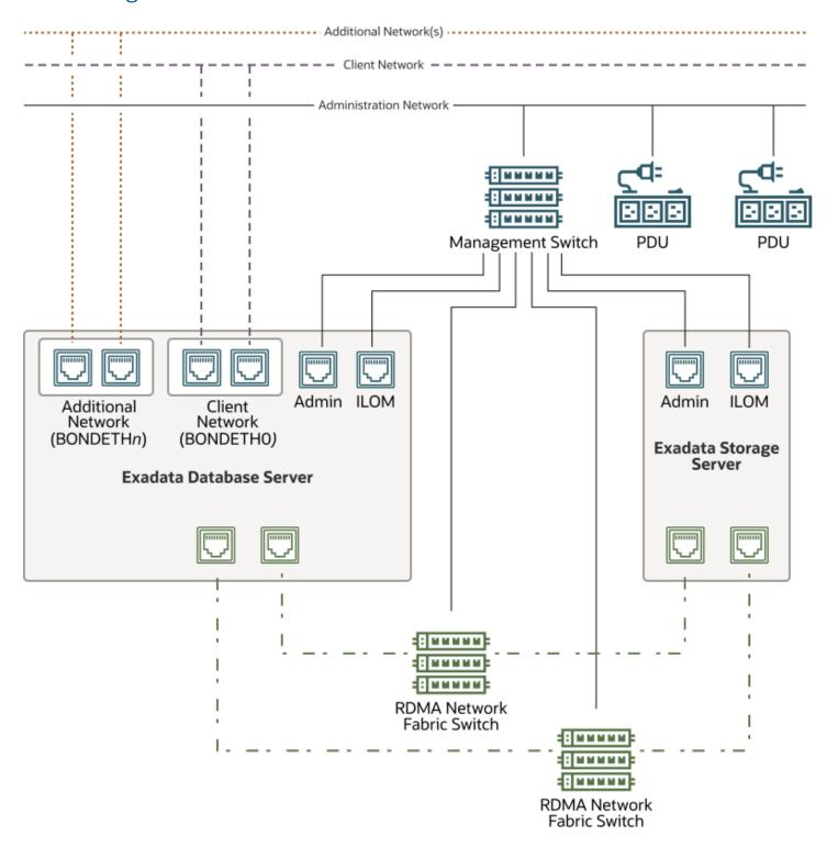
Oracle Exadata Database Machine includes equipment to connect the system to your network. The network connections allow clients to connect to the database servers and also enable remote system administration.
