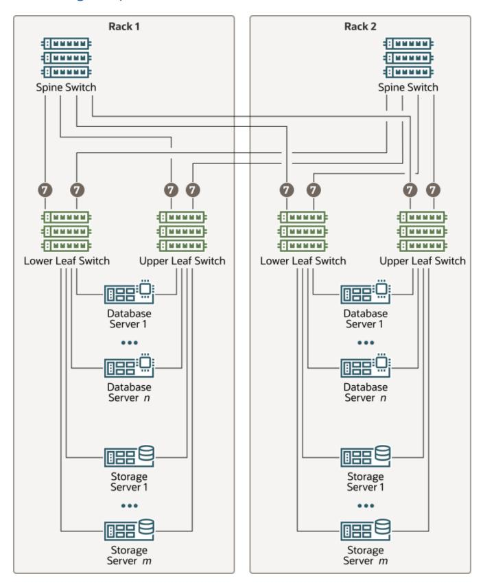
You can connect up to 12 RoCE-based Exadata racks together before external RDMA Network Fabric switches are required.
