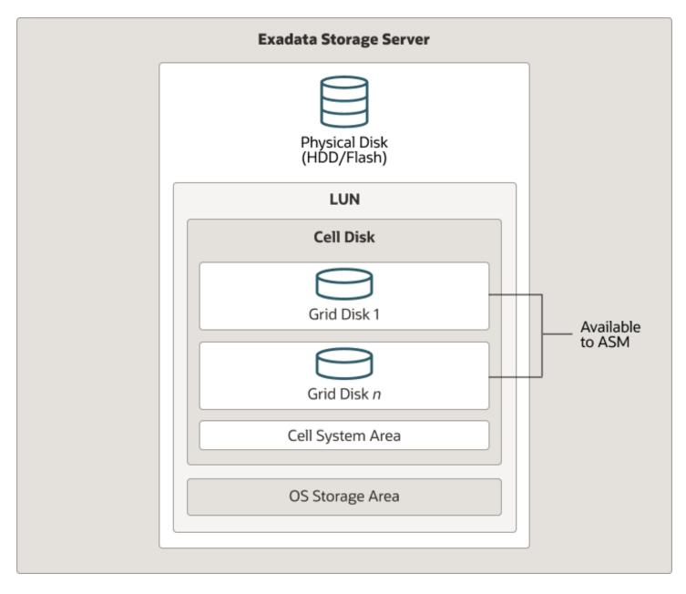
Oracle Exadata Storage Servers include physical disks, which can be hard disk drives (HDDs) or flash devices. Each physical disk has a logical address, called a logical unit number (LUN), which makes it available to the operation system (OS) and contains an OS storage area.
