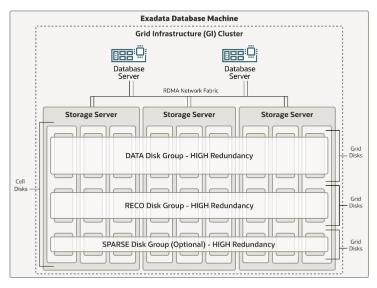
Oracle Exadata Database Machine uses Oracle Automatic Storage Management (Oracle ASM) as the cluster volume manager and file system to manage data storage.
