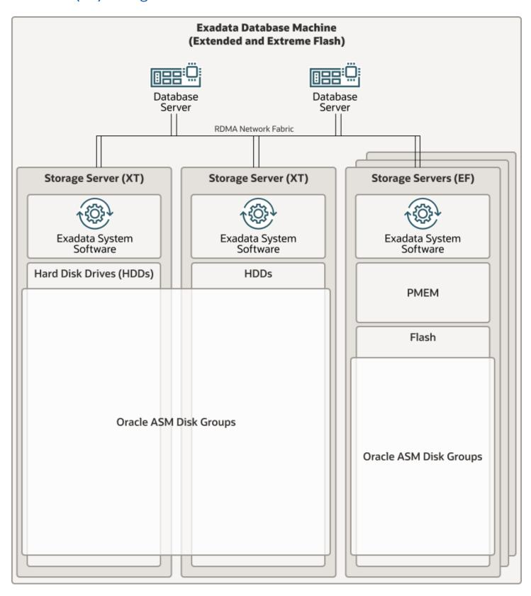
Each Oracle Exadata Storage Server Extended X9M-2 (XT) server includes twelve 18 TB hard disk drives (HDDs). Unlike Extreme Flash (EF) and High Capacity (HC) storage servers, XT servers don't contain flash or persistent memory (PMEM).
