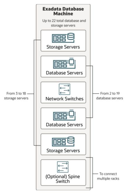
Oracle Exadata Database Machine features scale-out industry-standard database servers, scale-out intelligent storage servers, and high-speed internal RDMA Network Fabric that connects the database and storage servers.
