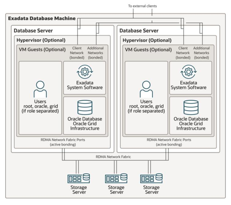
When deploying Oracle Exadata Database Machine, you can optionally implement virtual machines (VMs) on each database server. (Exadata Database Machine models with RDMA Network Fabric use Oracle Linux KVM. Earlier models that use Infiniband Network Fabric use Oracle VM.)
