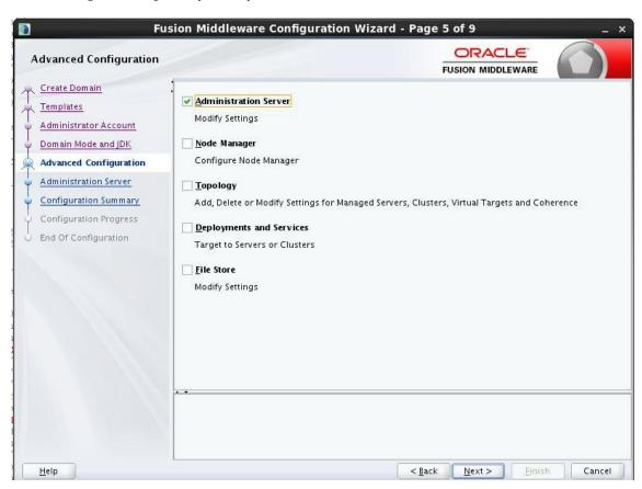
For the Administration Server a free port number must be specified. Enable SSL to support secure connections. An example using non default ports is shown below.
