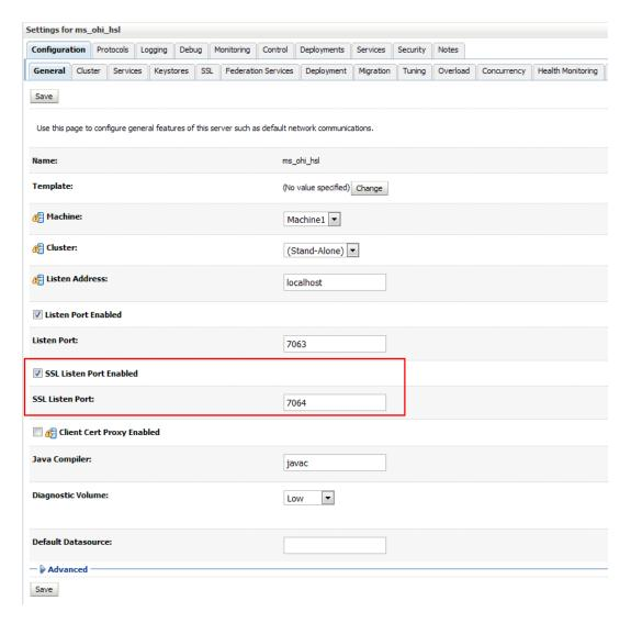
In previous versions of WebLogic, you needed to configure the Java Secure Socket Extension (JSSE) if the JDK version was below JDK 1.8.0\_162. Because the minimum JDK version for WebLogic 12.2.1.4.0 is JDK 1.8.0\_221, no further action is needed.
