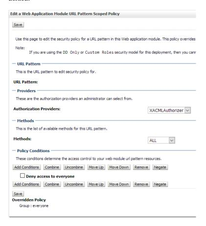
Note that the created policies survive an update of the ear-file but not a complete reinstall (deletion and subsequent installation of the ear-file). This allows for setting up policies as a one time configuration step and having all future updates adhere to the same (strict) set of policies.
