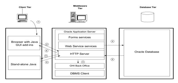
Fusion Middleware/Forms 12c introduced new ways to start and run a Forms application on the Client Tier.
