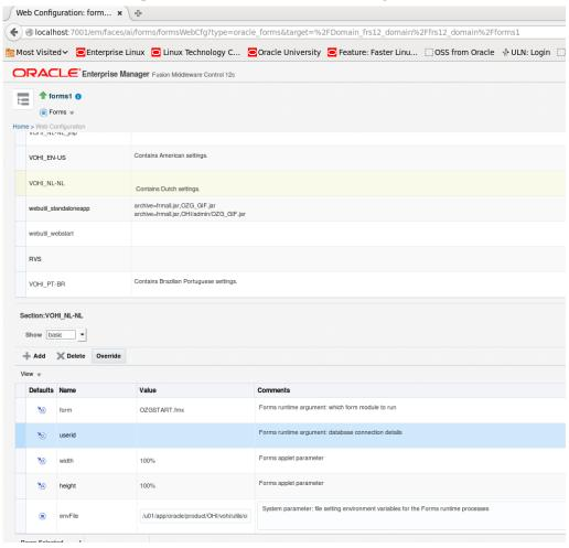
The <default> configuration will be inherited by all other configurations, so generic changes can be added over there. Specific configurations with different settings can be created to support different environment settings, for example to run with different colors, a different page title or other different characteristics as described later.
