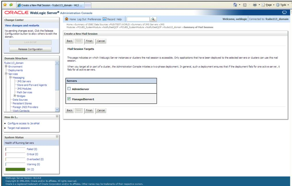
15. Check the box against the required servers and click 'Finish' to complete the configuration.
