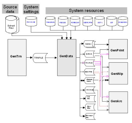
The GenData program uses the transaction list (TRNFILE) created by the GenTrn program as it processes the source data stored in the extract files. The FSISYS.INI file provides system setting information, such as whether or not it should stop processing if it encounters errors, how to identify key fields in extract files, whether or not it should check the output data size against the defined field length, and so on.
