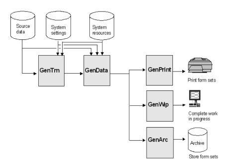
This illustration shows the main programs which make up Documaker Server and an overall view of the processing cycle.
