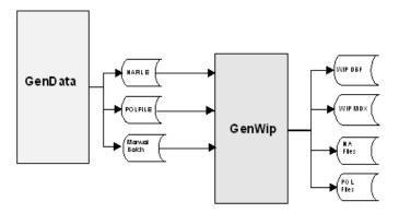
The GenWIP program receives information from the GenData program about incomplete transactions the GenData program found during its processing cycle. With this information, the GenWIP program creates files the WIP module of Documaker can read. Through the WIP module, data entry operators can complete the transactions by entering the missing information.
