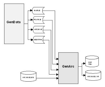
The GenArc program receives information from the GenData program, using many of the same files used by the GenWIP and GenPrint programs, such as the NAFILE and POLFILE. These two files identify the data to archive. The NEWTRN file tells the GenArc program where to find data in the NAFILE, which is created by the GenArc program.
