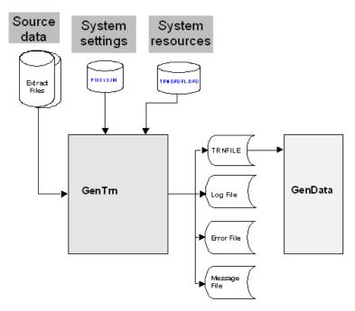
The GenTrn program takes the source data, which is stored in extract files, and creates a list of the transactions, which is stored in the TRNFILE, or transaction file. This transaction list is then used by the GenData program as it processes the transactions.
