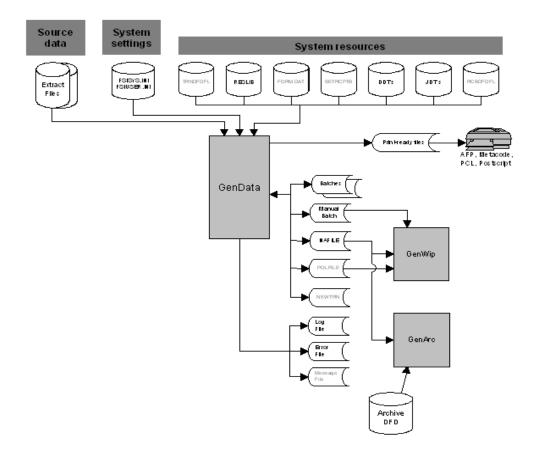
As shown in the illustration above, the GenData program processes transaction records, originated from the source data, and creates various output files for print, WIP or GenArc. By combining the functions of GenTrn and GenPrint into GenData, you reduce the number of times the system needs to open and close files, thus enhancing the overall performance of your system.
