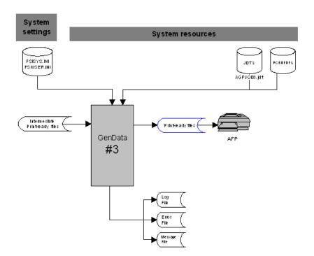
The third execution of GenData uses the AFGJOB3.JDT file. This JDT file uses base and form set rules shown in this example to merge data intermediate print-ready files into a print-ready file for an AFP printer.
