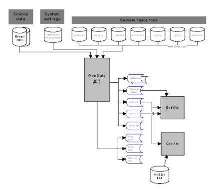
The first execution of GenData uses the AFGJOB1.JDT file with the base and form set rules shown in this example to create output files shown in the illustration.
