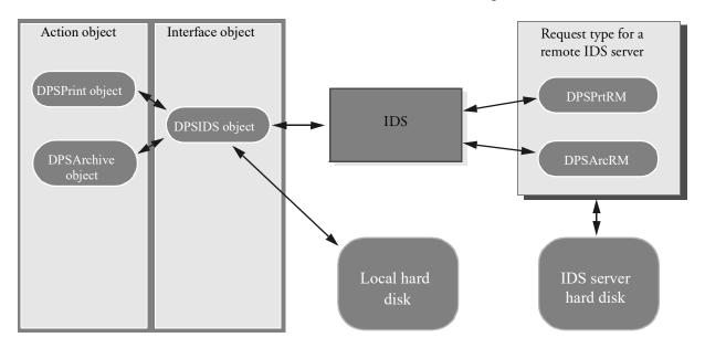
This illustration shows how it works with IDS running on a different machine:
