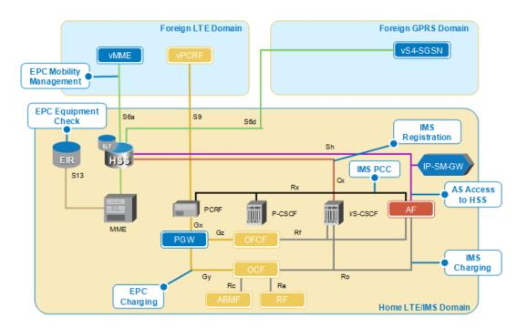
Figure 1-1 Selected Diameter Interfaces in LTE and IMS
