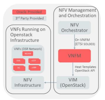
DSR application automatic instantiation process includes two operations specified by the ETSI NFV SOL 003. Those operations supported by DSR VNFM currently are as follows:
