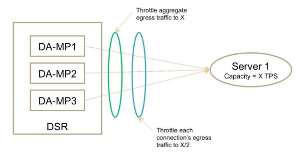
Figure 2-22 DSR Aggregate and Per-Connection Egress Throttling
