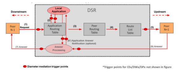
The mediation framework also supports defining multiple mediation rules at a single trigger point or invoking the same mediation rule at multiple trigger points.
