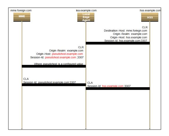
Figure 2-47 S6a-S6d HSS Topology Hiding CLR Message Flow
