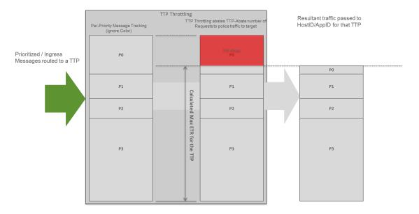
Figure 2-30 Throttle by Message Priority Only when support for 5 message priorities is enabled
