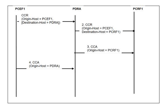
n the CCR-I, the PCEF optionally includes the Destination-Host of P-DRA and upon receiving an initial CCA from the P-DRA, populates the Destination-Host AVP with the P-DRA ID for subsequent messages (CCR-U and CCR-T). This is based on the Origin-Host AVP received in the initial CCA from the P-DRA.
