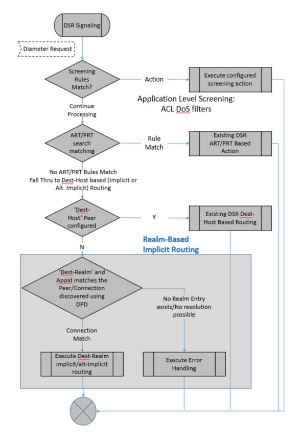
Figure 2-14 High Level DSR Routing Flow – Fall through to Dest-Realm Based Implicit Routing
