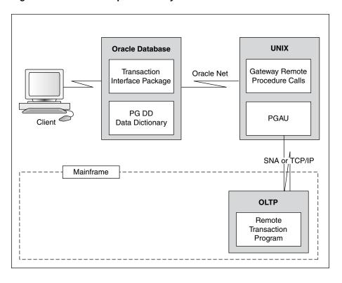
Figure 1-1 Relationship of Gateway and the Oracle Database
