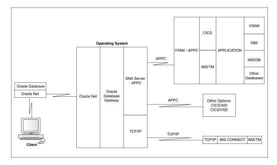
Figure 1-2 Gateway Architecture Featuring SNA or TCP/IP Protocol
