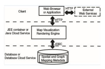
Figure 1-1 Map Visualization Component Architecture
