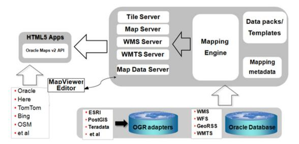
Figure 2-15 Architecture for Oracle Maps Applications
