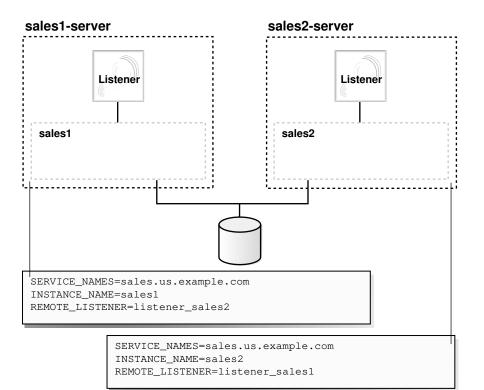
Figure 13-3 Load Balancing Environment for a Dedicated Server Configuration
