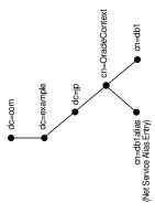
There are several uses for network service aliases. As shown in Figure 3-9, a network service alias can be useful as a way for clients to refer to a network service name by another name. Another use is to have a network service alias in one Oracle Context for a database service or network service name in a different Oracle Context. This enables a database service or network service name to be defined once in the directory server, but referred to by clients that use other Oracle Contexts.
