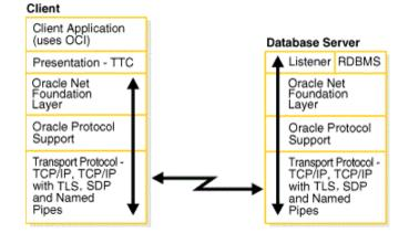
Figure 5-1 Layers Used in an Initial Connection
