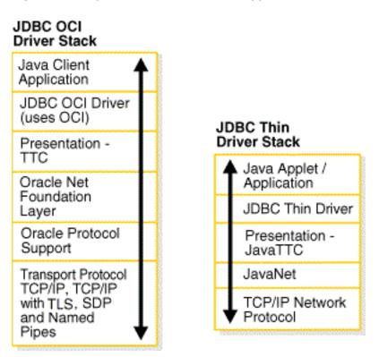
Figure 4-3 Layers Used for Java-Client Applications
