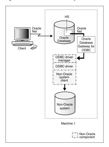
Figure 1-2 Oracle and Non-Oracle Systems on the Same Machine
