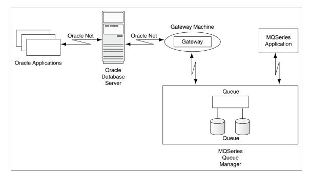
Figure 1-1 Components of the Gateway Architecture
