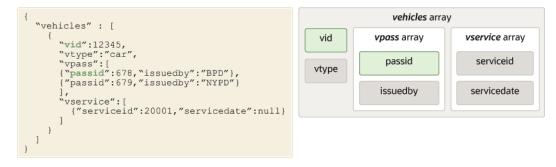
The following is an example of a composite multikey index in which fields of an array and fields of an inner array are used together, however, notice that the immediate parent array of the two fields are not the same. The following is an invalid index creation statement. The index is being created on the passid and serviceid fields in the vehicles array in the UserInfo table. Note that within the vehicles array, passid is inside the vpass array, and serviceid is inside the vservice array.
