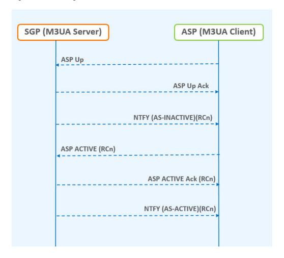
Figure 2-3 Message Flow for ASP - M3UA Client
