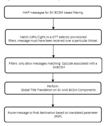
Figure 2-15 Call Flow for Opcode-Msisdn Based Filtering
