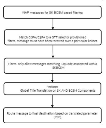
Figure 2-16 Call Flow for SK BCSM Based Filtering
