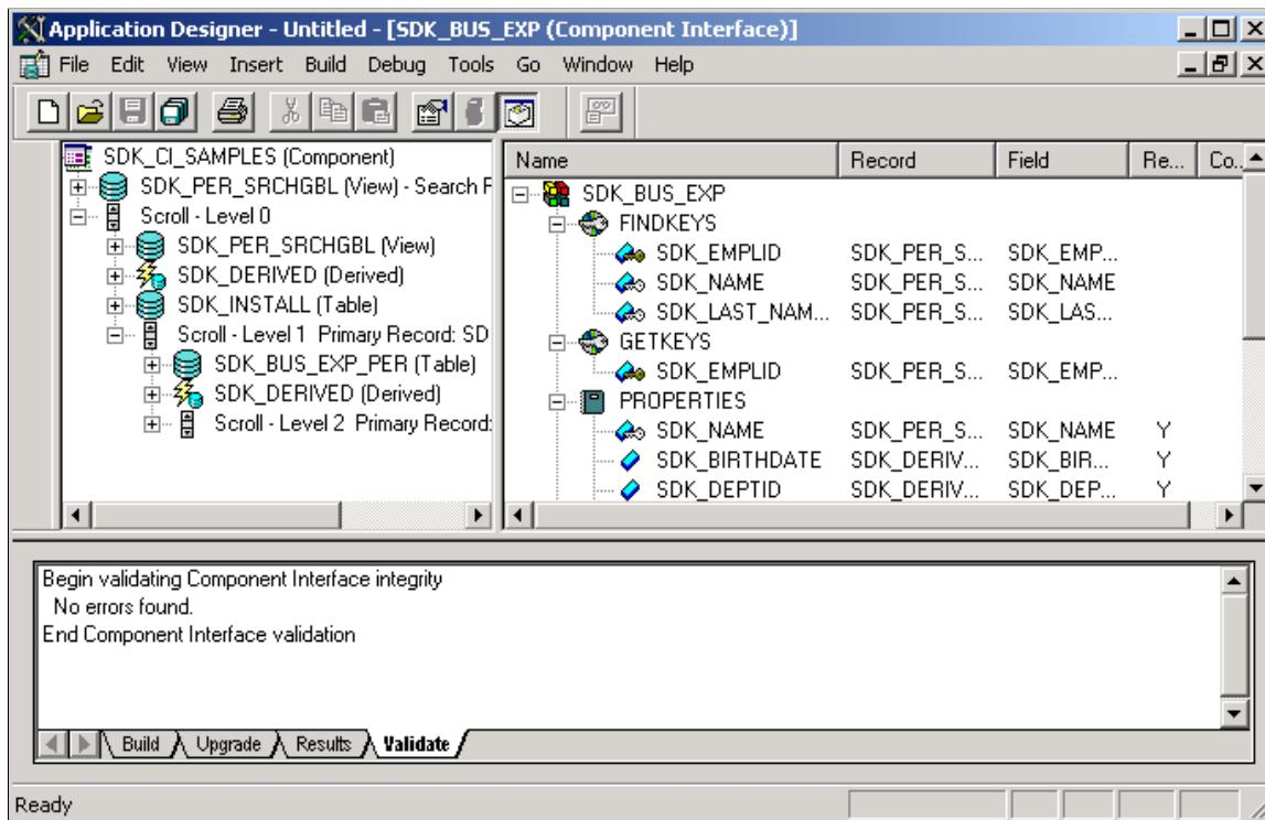
The component view shows records and scrolls in the component, using a tree representation. The structure is the same as the one you see on the structure tab of a component in PeopleSoft Application Designer. Drag the fields and collections that you want exposed to the component interface view.
