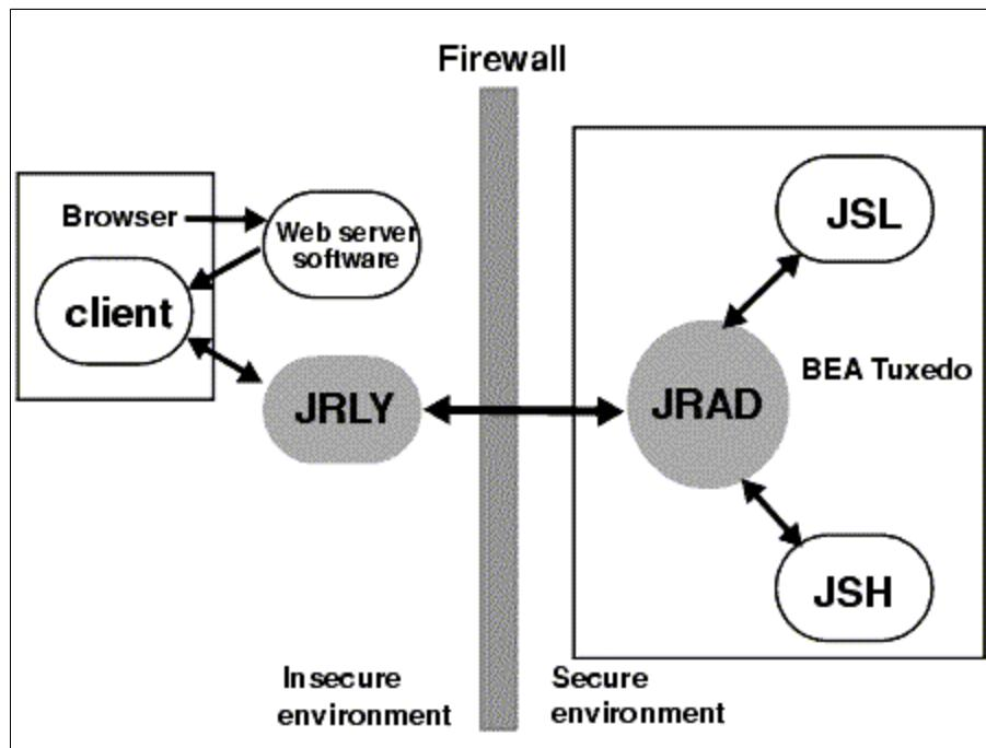
Jolt Internet Relay consists of two elements: Jolt Relay (JRLY) and Jolt Relay Adapter (JRAD). It's important to understand the difference between these two elements.
