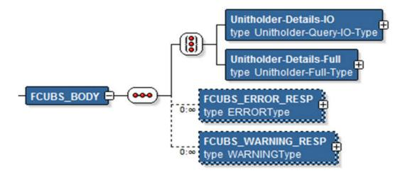
FCUBS\_BODY will contain additional nodes for error response and warning response. A diagrammatic representation of the Error response is as shown below:
