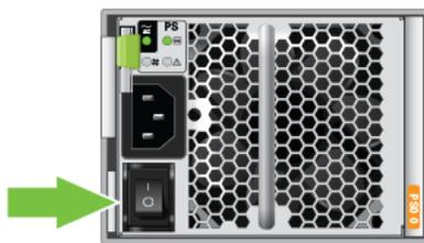
4. Press the Power button located on the front of the first (bottom) management node. See [Figure 5.5](#).
