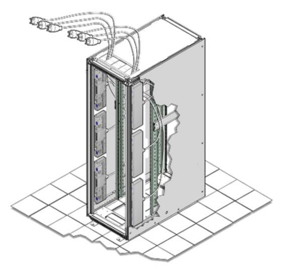
Plug the power distribution unit (PDU) power cord connectors into the facility receptacles. Ensure the breaker switches are in the OFF position before connecting the power cables.
