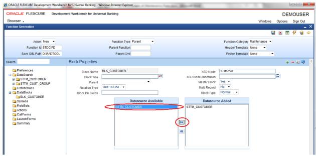
Fig 12.10: Attaching Data Sources to Data Block
