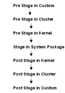
Fig 12.31: Flow of control through Hook Packages
